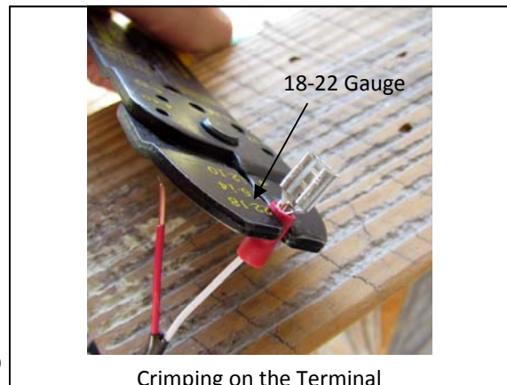
Crimping on the Terminal
