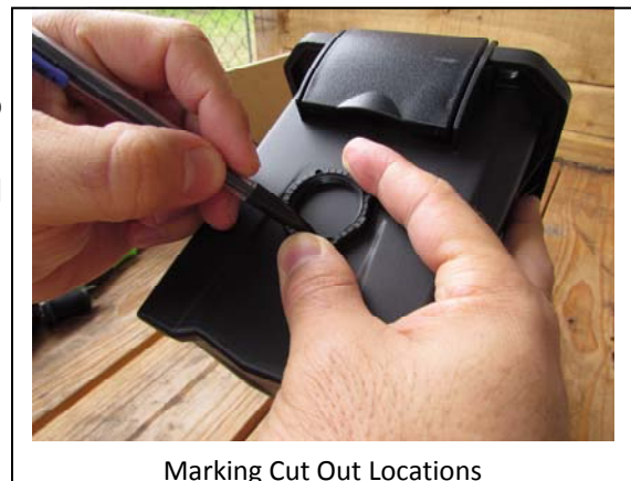
Marking Cut Out Locations
